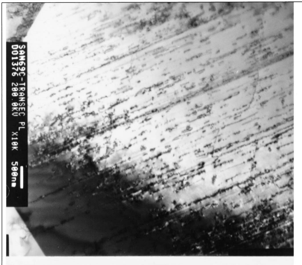
Figure 4 Dislocation structures in the Alloy 690 material fatigue-tested with 0.2% total strain amplitude at 204°C, N = 40000 cycles.
